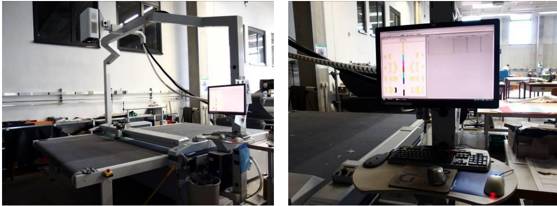
Fig. 25 and 26: Dieless cutting table (oscillating knife)
