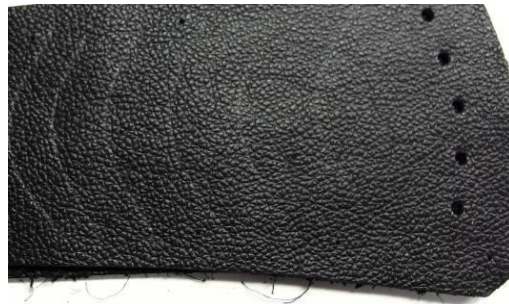
Fig. 20 and 21: Cutting dies can be equipped with punchers, prickers, or markers, which can make subsequent work steps redundant
