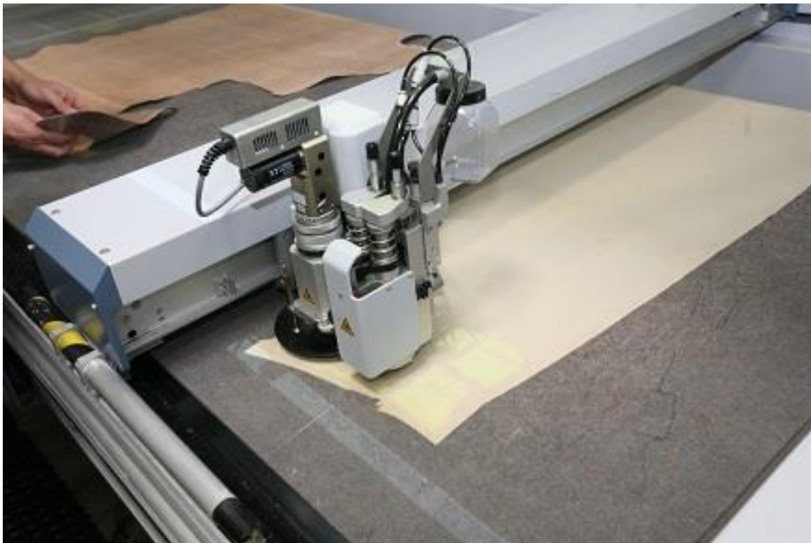
Fig. 2: CAD cutting table with projection and oscillating knife
